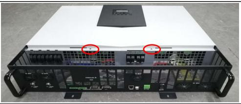
Open the top cover and check the first cable in the figure, is it well connected?
